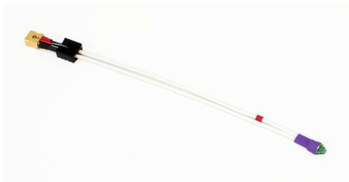
TriMode™ Long Reach Solder Tip (0 \Omega tip resistor) A high performance solder tip for use with memory chip interposers with embedded 175 \Omega resistors. Up to 20 GHz bandwidth.
